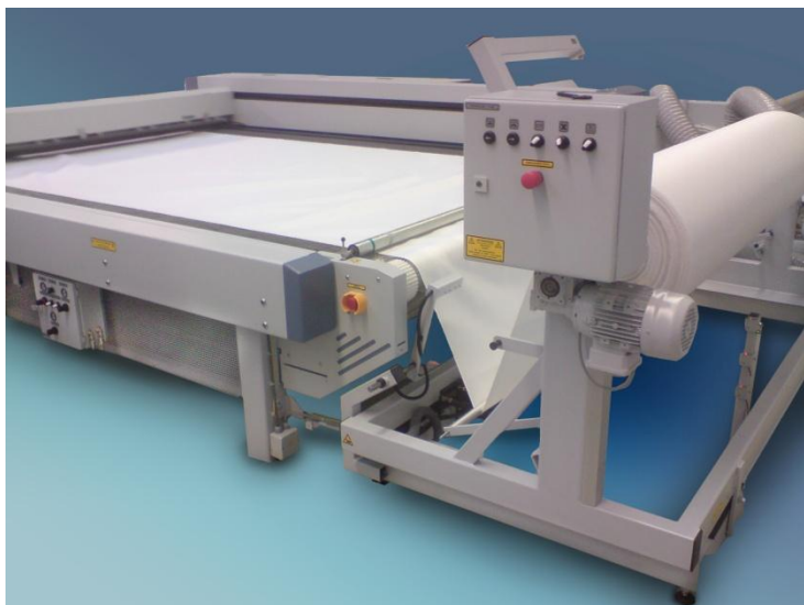
Feeder with driven unwinding shaft , with loop control for tension free supply of delicate fabrics.
