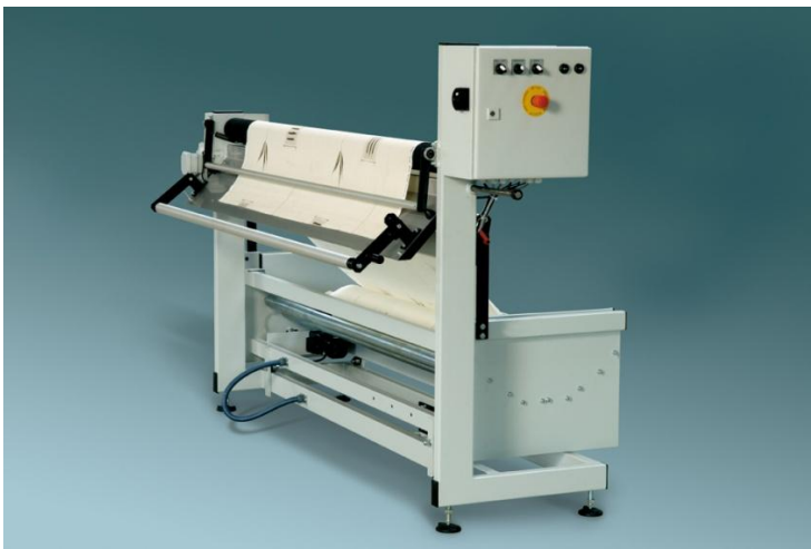
Cradle feeder for fabrics, with transport roller, dancer, edge control, and reverse system.
